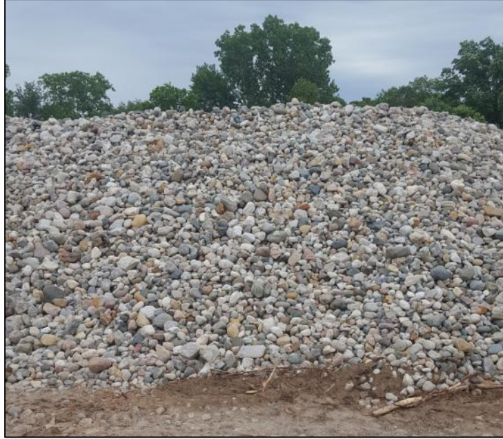
Figure 4.2. Coarse alluvium gradation example
